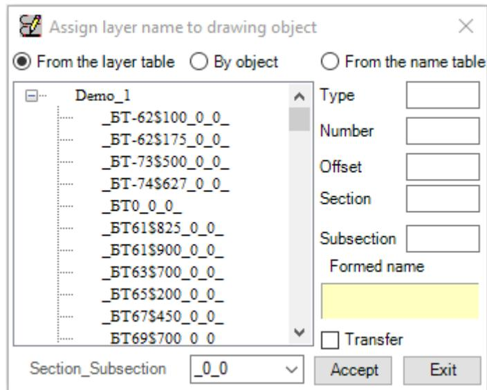
**Figure 214.** Assign layer name to drawing object dialog box
