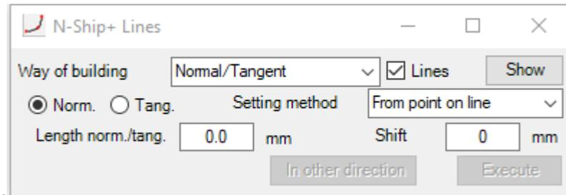
**Figure 66.** Dialog box for the method of specifying from a point on a line
