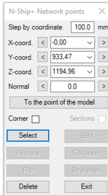
**Figure 31.** Network Points window when selecting a single point
