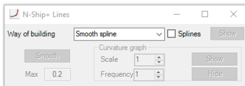
**Figure 62.** The dialog box for the **Smooth spline** method
