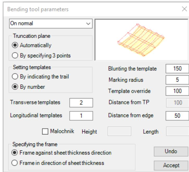
**Figure 160.** Bending tool parameters dialog box
