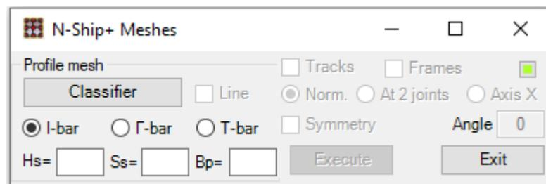
**Figure 98.** Dialog window with parameters for building the profile mesh
