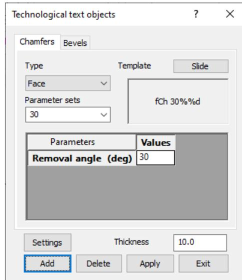
Pic. 88. Window for creation of technological texts, tab **Chamfers**
