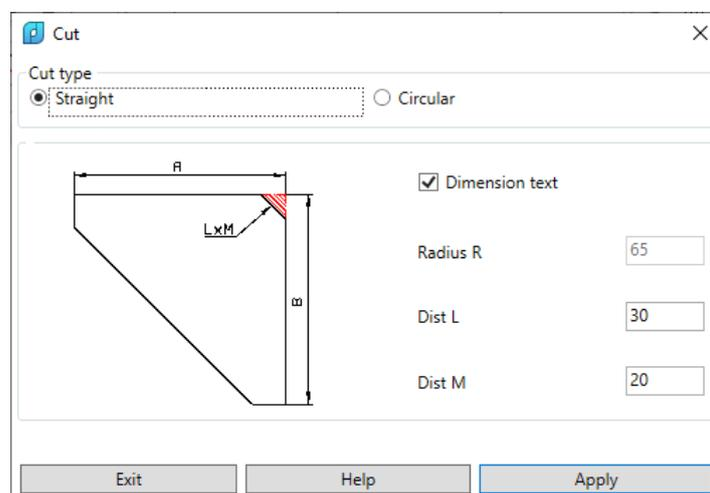
Pic. 44. Straight cut parameters
