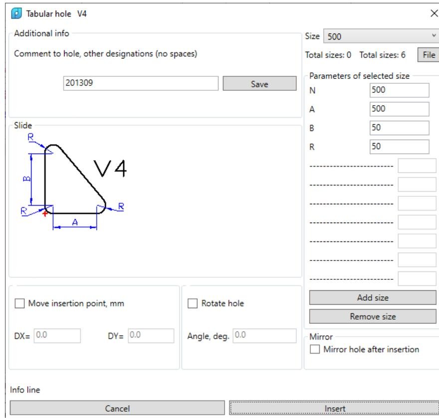
Pic. 55. Window for setting parameter values for the hole type size
