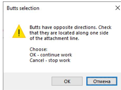
Pic. 29. Warning for suspicious input of second point for butt 2
