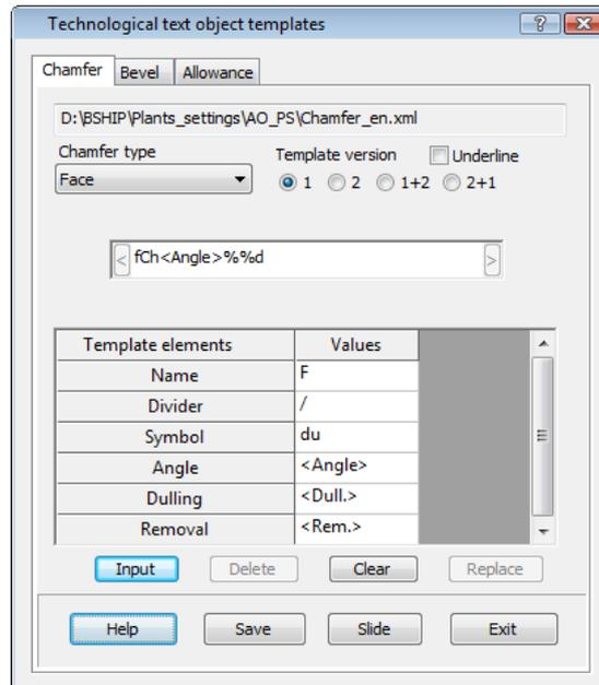
Pic. 94. Dialog box for tuning templates of chamfers, bevels and allowances
