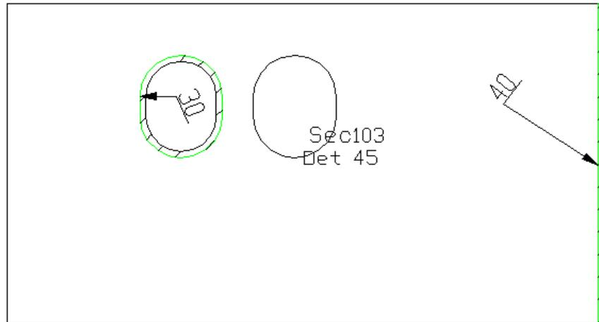
Pic. 101. Sample of allowances to part contour fragment and to inner hole
