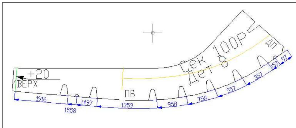
Pic. 67. Sample dimensioning lengths along curve up to holes
