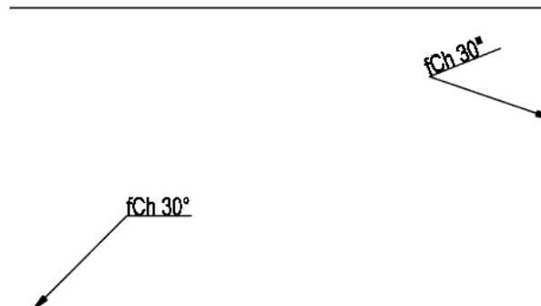
Pic. 89. Sample chamfers
