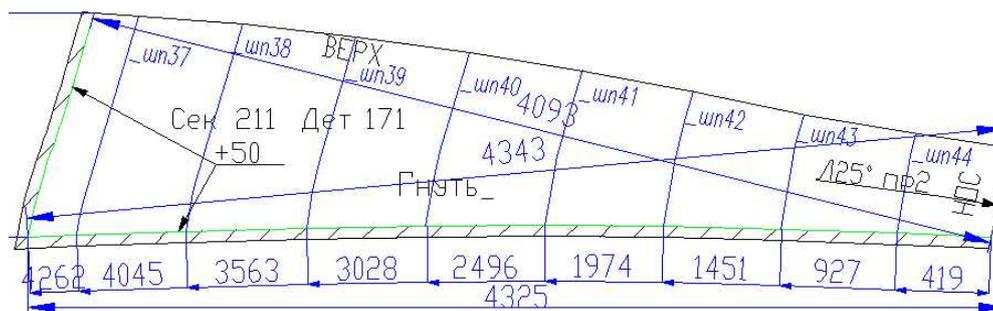
Pic. 68. Sample dimensioning lengths along curve up to girders
